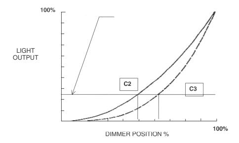
Our eyes are most sensitive to low luminous intensity, in particular to the range that lies below 25% of maximum luminous intensity (100%). Therefore, using C3 yields a more flexible control range.
