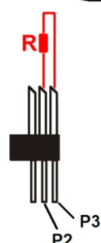
How to turn the controller line from 3-pins into 5-pins (plug and socket).
